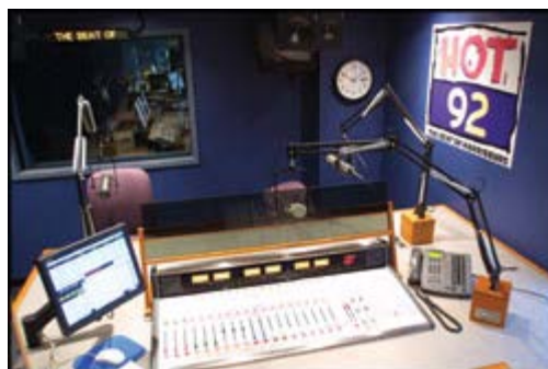
Like the WWKL studio shown here, all the studios have low equipment profiles to maintain easy sight lines.
